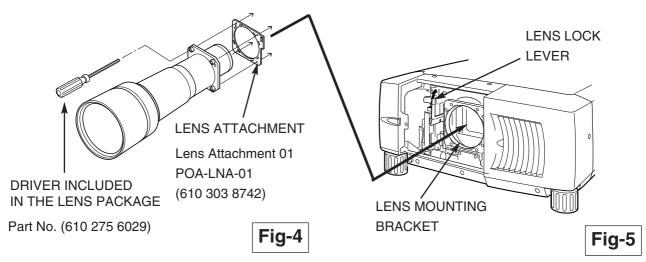
Grasp (release lock) the Lens Lock Lever and turn it fully upward. (See Fig. 6)
